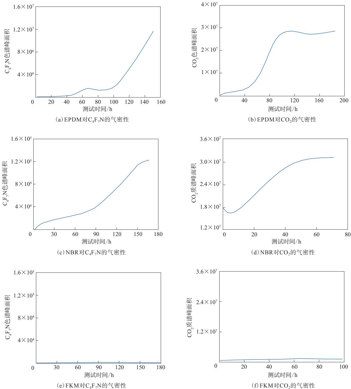
图2 3种橡胶材料对 $\text{C}_4\text{F}_7\text{N}$ 和 $\text{CO}_2$ 的气密性测试结果Fig. 2 Air tightness test results of three rubber materials to  $\text{C}_4\text{F}_7\text{N}$  and  $\text{CO}_2$
